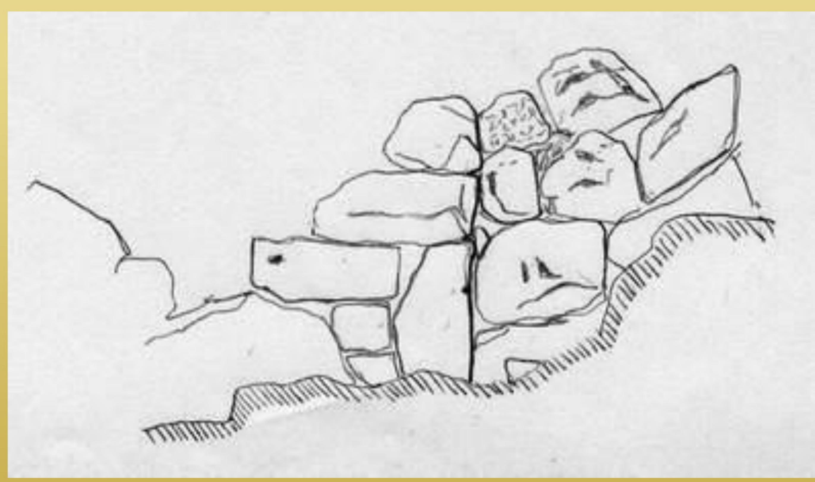
Sketch of the inner front of the south wall at the location highlighted by the small arrow in figure 2. The three stones vertically aligned suggest existence of an interruption in the stonework that could be related to an opening (e.g. door) or to cornerstones (sketch by G. Pesce)
